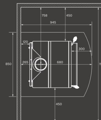
All dimensions and clearances are in mm. Clearances are with factory flue shield.
