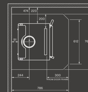
All dimensions and clearances are in mm. Clearances are with factory flue shield.
