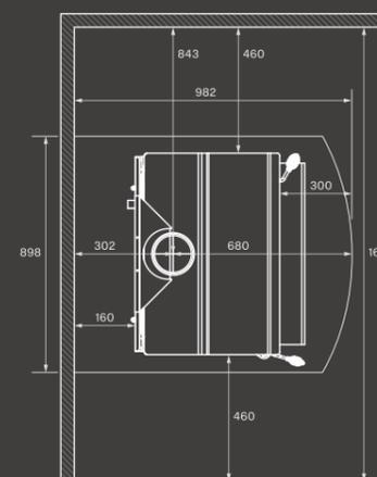
All dimensions and clearances are in mm. Clearances are with factory flue shield.
