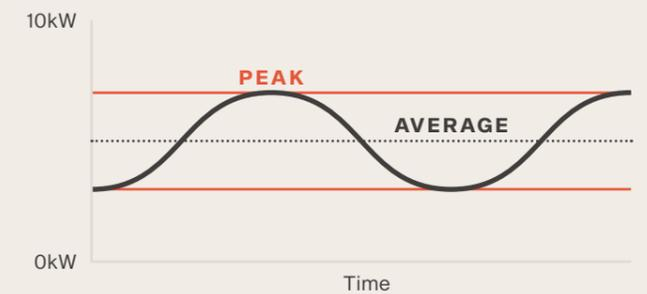
While some brands represent their outputs at 'Peak', which is the very top of the heating curve, we prefer to show an accurate representation of a fire's true performance over time.
