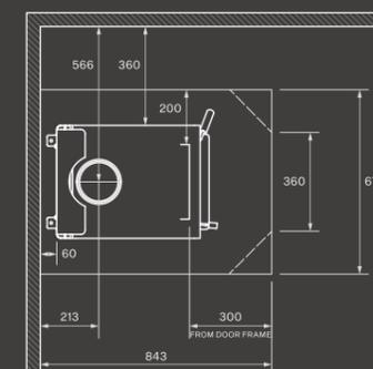
All dimensions and clearances are in mm. Clearances are with factory flue shield.
