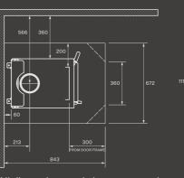
All dimensions and clearances are in mm. Refer to installation manual Clearances are with factory flue shield.
