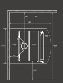
All dimensions and clearances are in mm. Refer to installation manual Clearances are with factory flue shield.
