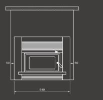
All dimensions and clearances are in mm. Refer to installation manual Clearances are with factory flue shield.
