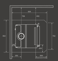
All dimensions and clearances are in mm. Refer to installation manual Clearances are with factory flue shield.
