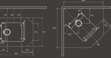
All dimensions and clearances are in mm. Refer to installation manual Clearances are with factory flue shield.
